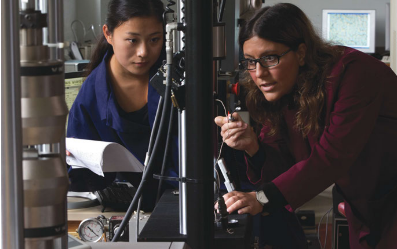
Master's candidate Yuwei Zhai and Professor Lados inspect an aluminum sample undergoing a test in a machine that can stretch metal until it breaks. Knowledge gained by testing alloys can lead to better computational tools and greater use of light metals in cars, trucks, and airplanes.
